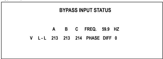
The Bypass Input Block displays the following real-time data:
